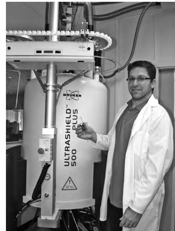
TRU Faculty Bruno Cinel, with the 500 MHz Nuclear Magnetic Resonance (NMR) Spectrometer
