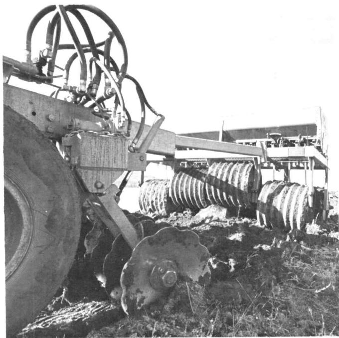
Fig. 2. Rangeland disc-seeder developed and used by the British Columbia Ministry of Agriculture.
