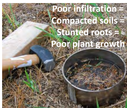
Figure 1 and 2 (Above). Pictures of the infiltration test (above left) and an soil sample with good aggregation (above right).
