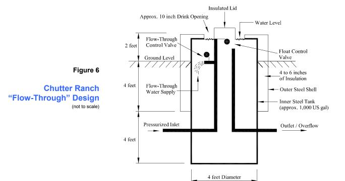
Note this trough has heat supplied with flow-through water combined with wall insulation and small water surface area for reduced heat losses. It may be used as a float controlled waterer or as a flow-through one. **Random Pointers** The following are a few pointers for winter watering systems.
