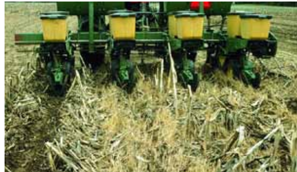
Figure 1. No-till seeding into a chemically killed rye cover crop
